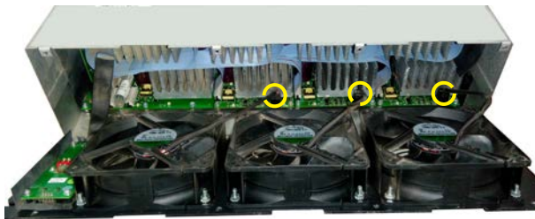
Figure 3: Disconnect the fan wires
